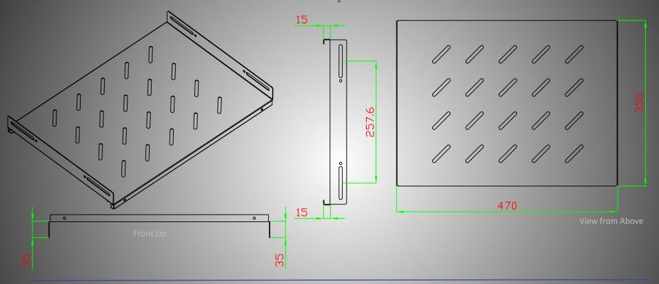
This shelf can be installed in all All-Rack 600mm deep floor cabinets. It has been specifically designed to fix at the front and rear.
