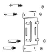
4 Install the bracket to the pre-installed plate
