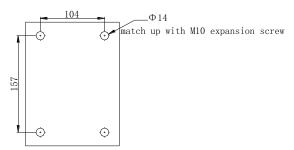
3 Fix the pre-installed plate
